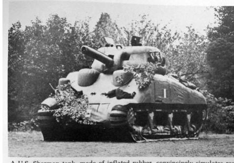
A US Sherman tank made of inflated rubber convincingly simulates real
